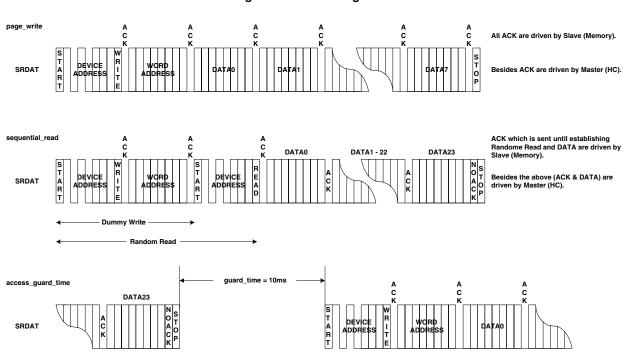
Figure 8-2. I<sup>2</sup>C Timing Chart
