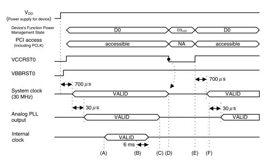
Figure 6-3. Clock Operation Diagram (Using 30 MHz Crystal)
