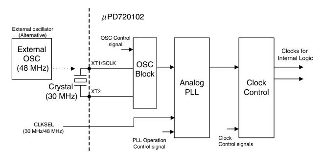
Figure 6-2.  $\mu$ PD720102's Clock System
