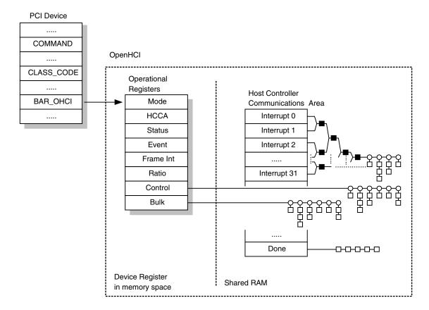
Figure 3-1. OpenHCI's PCI Configuration Space
