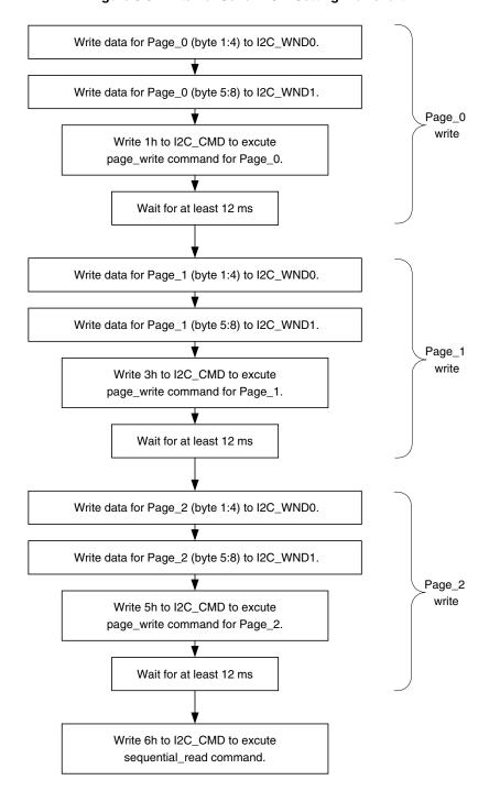
Figure 8-3. External Serial ROM Setting Flowchart
