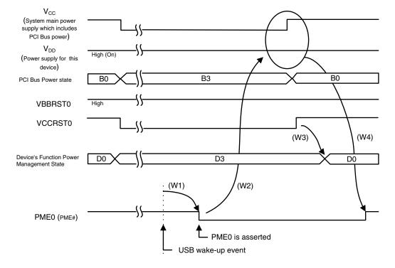
Figure 6-1. Wake Up State Transition from D3cold
