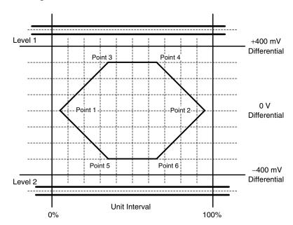
Figure 10-4. Transmit Waveform for Transceiver at DP/DM
