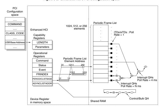
Figure 3-2. Enhanced HCI's PCI Configuration Space
