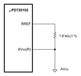
Remark The board layout should minimize the total path length from RREF through the resistor to AVss(R) and path length to AVss (analog ground). AVss must be stable.
