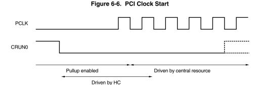
HC may require the PCI clock to complete current internal processes. At that time, HC will assert CRUN0 for two successive clocks after it has been deasserted.
