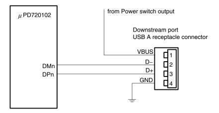
Figure 9-1. USB Downstream Port Connection
