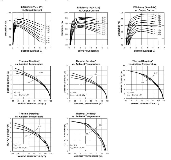
**Die Temperature\***: The temperature measurement was taken at the hottest point on the MIC26400 case mounted on a 5 square inch 4 layer, 0.62", FR-4 PCB with 2oz finish copper weight per layer, see Thermal Measurement section. Actual results will depend upon the size of the PCB, ambient temperature and proximity to other heat emitting components.
