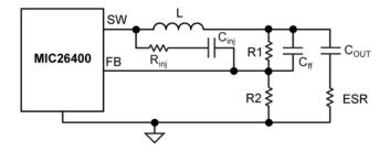
Figure 5c. Invisible Ripple at FB
