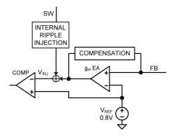
Figure 7. Internal Ripple Injection
