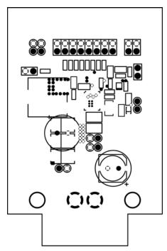
Figure 10. MIC26400 Evaluation Board Mid-Layer 1 (Ground Plane)
