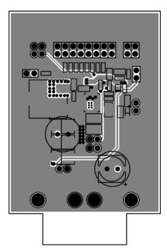
Figure 11. MIC26400 Evaluation Board Mid-Layer 2
