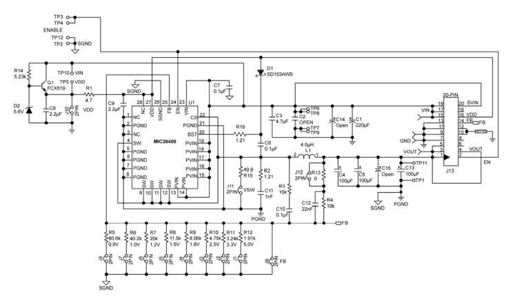
Figure 8. Schematic of MIC26400 Evaluation Board (J13, R13, R15 are for testing purposes)
