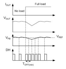
Figure 3. MIC26400 Load Transient Response
