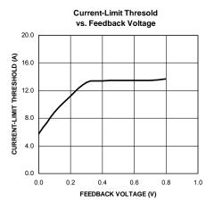
Figure 4. MIC26400 Current Limit Foldback Characteristic
