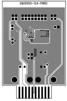
Figure 12. MIC26400 Evaluation Board Bottom Layer
