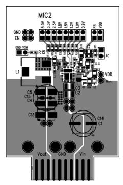
Figure 9. MIC26400 Evaluation Board Top Layer
