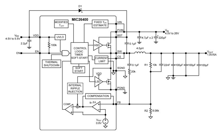
Figure 1. MIC26400 Block Diagram
