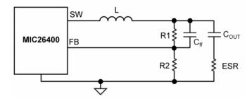
Figure 5b. Inadequate Ripple at FB
