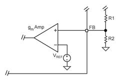
Figure 6. Voltage-Divider Configuration
