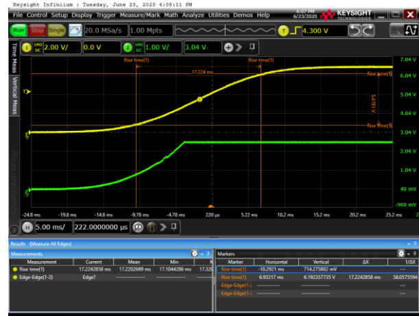
Figure 8. Power Up, 15 ms, V_{BIAS} = 6.5\text{ V} , R_{BIAS} = 2.5\text{ k}\Omega
