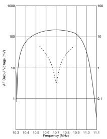
Input = 100dBµ fdev. = ±80kHz fmod. = 1kHz Vcc = 3.0V
