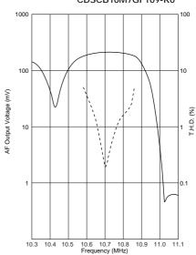
$\begin{aligned} &\text{Input} = 100 \text{dB}\mu \\ &\text{fdev.} = \pm 64 \text{kHz} \\ &\text{fmod.} = 1 \text{kHz} \\ &\text{Vcc} = 3.0 \text{V} \end{aligned}$
