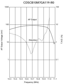
$\begin{array}{l} Input = 100 dB \mu \\ fdev. = \pm 60 kHz \\ fmod. = 1 kHz \\ Vcc = 3.0 V \end{array}$
