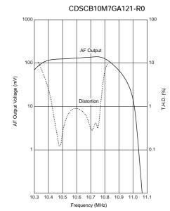
$\begin{array}{l} Input = 100 dB\mu \\ fdev. = \pm 75 kHz \\ fmod. = 1 kHz \\ Vcc = 3.2 V \end{array}$
