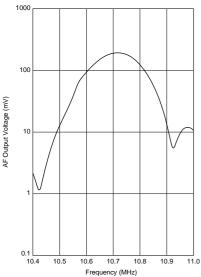
$\begin{array}{l} \text{Input} = 100 \text{dB} \mu \\ \text{fdev.} = \pm 50 \text{kHz} \\ \text{fmod.} = 1 \text{kHz} \end{array}$ Vcc = 5.0V
