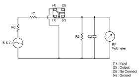
C2=10pF (Including stray capacitance and Input capacitance of RF Voltmeter) E1 : S.S.G. Output Voltage
