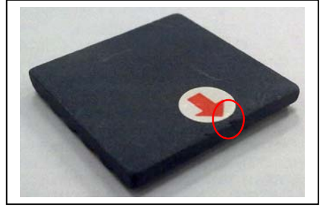
Appearance Description : Hole Limitation : Less than 2mm
