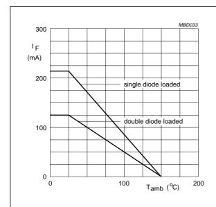
Device mounted on an FR4 printed-circuit board.
