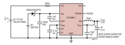
Figure 11. 5V to 16V Solar-Powered 2.5V Supply with Supercapacitor for Increased Output Energy Storage and Battery Backup
