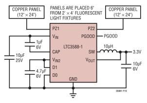
Figure 10. Electric Field Energy Harvester
