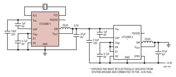
Figure 13. Piezoelectric Energy Harvester with ±3.3V Outputs
