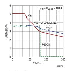
Figure 2. PGOOD Operation During Transition to UVLO
