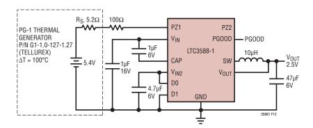
Figure 12. Thermoelectric Energy Harvester
