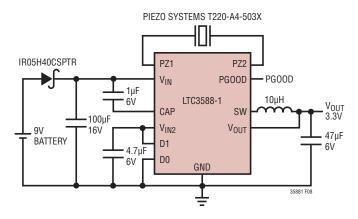
Figure 8. Piezo Energy Harvester with Battery Backup
