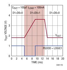
Figure 3. PGOOD Operation During DO/D1 Transition
