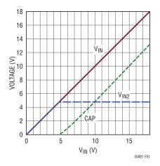
Figure 1. Ideal V<sub>IN</sub>, V<sub>IN2</sub> and CAP Relationship
