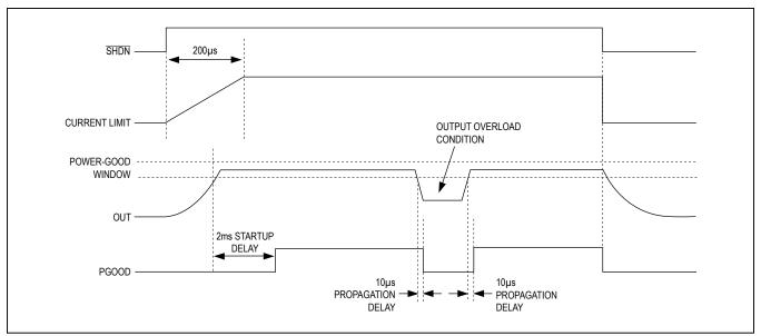
Figure 3. MAX8794 PGOOD and Soft-Start Waveforms
