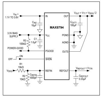
Figure 1. Standard Application Circuit
