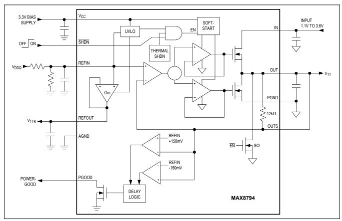
Figure 2. Functional Diagram
